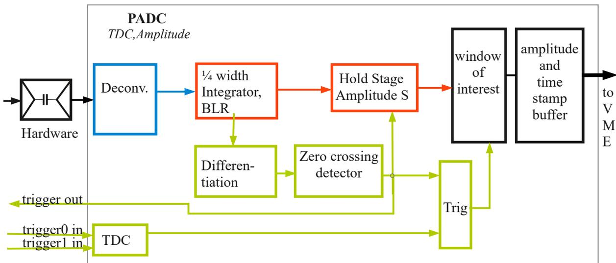
The signal is amplified filtered digitized. Then the pre- differentiation is removed by a deconvolution. Then the signal is integrated with a time constant of about  $\frac{1}{4}$  of the FWHW of the signal. This improves the resolution to up to  $\frac{1}{32000}$  of the full range.
