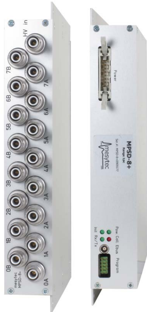
Standalone housing of MPSD-8+ in NIM case with mounting flaps
